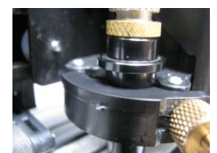
Figure 72: Installing the blade assembly
